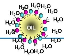
Droplets of oil, in water, stabilised with surfactant
